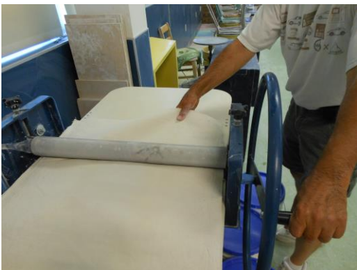
Pulling on canvas at the same time you turn the large rolling handle
