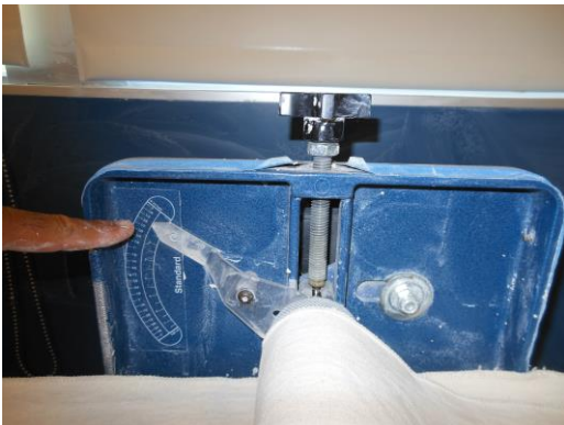
Thickness indicator and adjusting screws
