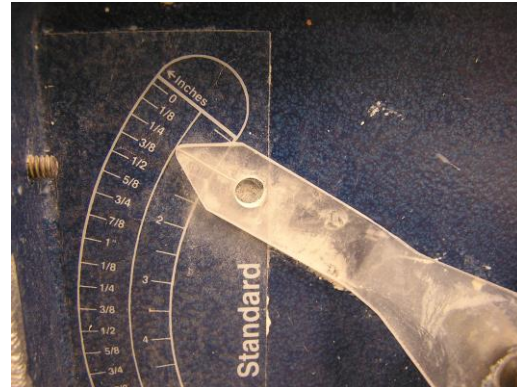
Thickness indicator and adjusting screws
