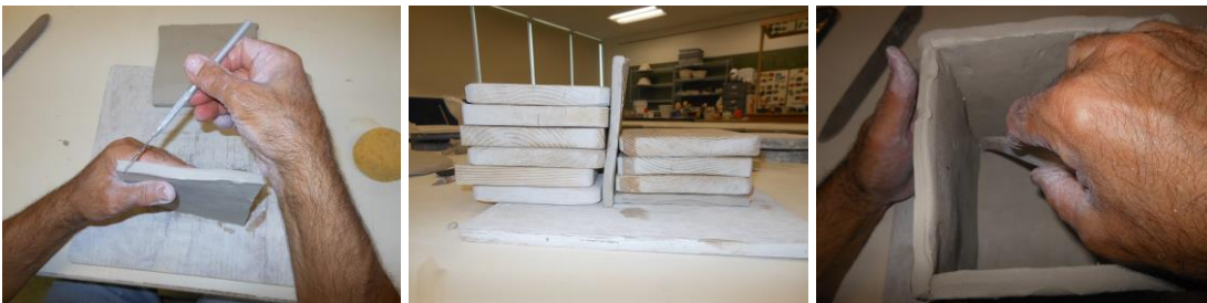
Two surfaces being joined Holding first wall in place as you add more walls. Compressing the joints.
