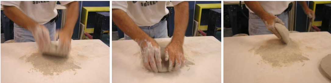
Throwing the clay onto the wedging table and getting it ready for the slabbing machine
