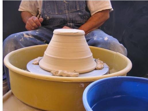
Picture of smooth walls. Wheel is spinning fast enough to get smooth walls
