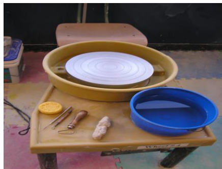
Tools needed for trimming sitting on a wheel with small slug of clay
