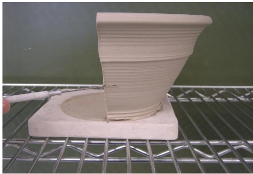
Bowl cut in half with needle tool marking the walls where they begin to get thick
