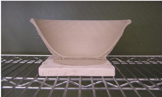
Untrimmed bowls cut in half showing (with hash marks) what will be trimmed off
