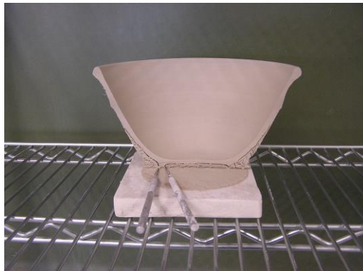
Bowl cut in half with needle tools showing where to make the two marks
