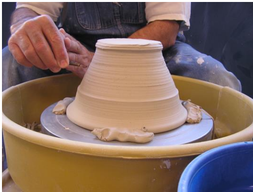
Small trimming tool at a 90 degree angel to the bowl (NO).
